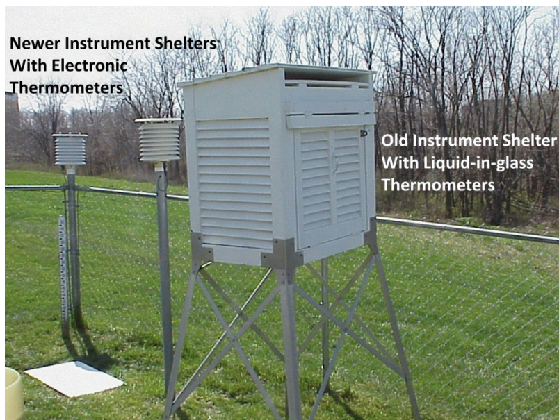
Fig. 5. Surface temperature measurements have changed. A comparison of the wooden Stevenson shelters that used to house traditional liquid-in-glass thermometers, versus the newer enclosures which now contain electronic thermometers (thermistors).
