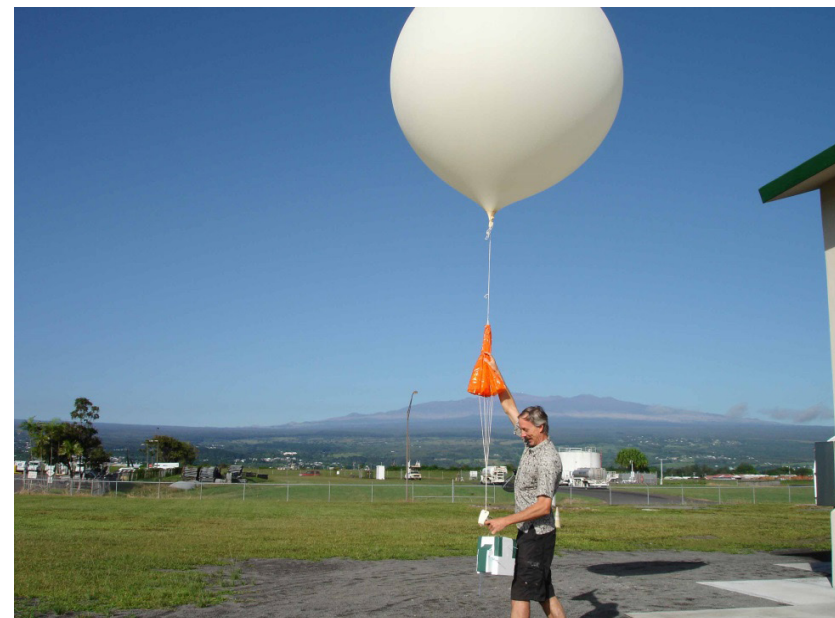
Fig. 6. A radiosonde (weather balloon) instrument package ready to be launched at Hilo, Hawaii, to measure the temperature profile of the lower atmosphere.
